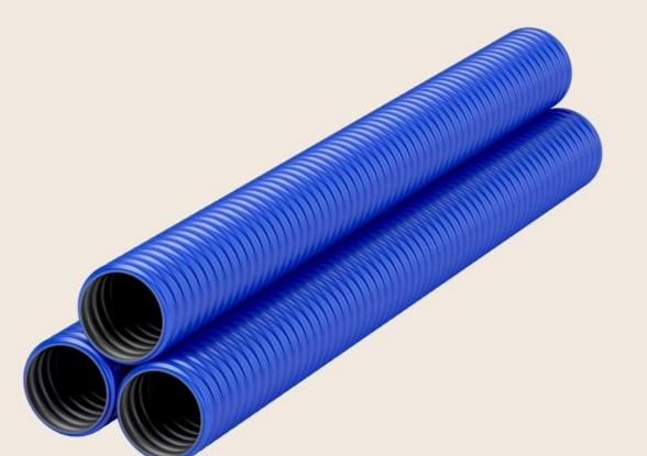
The material used to create double wall corrugated (DWC) pipes is high-density polyethylene (HDPE). They feature a smooth inner wall and an outside wall with corrugations. The pipe's corrugations provide it strength and stiffness, and its smooth inner wall improves water flow. The sizes, lengths, and thicknesses of DWC pipes vary.
